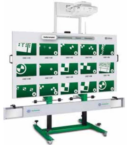
a precise location in relation to the camera being calibrated. The ECU interprets the image and, via software, makes any pitch, roll or yaw adjustments required to ensure the camera looks precisely where required. This sets a base for the system to calculate where a relevant obstacle is in relation to the vehicle.
