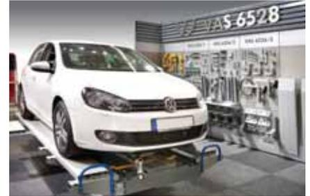
few seconds to set up and it has a convenient draw aligner that can be turned 180 degrees around the platform at one end and tilted 90 degrees horizontally. Once pulling begins, the draw aligner finds the correct position. For more pulling power, there is the Speed Plus bench, which allows the attachment of two draw aligners, one at either end.
